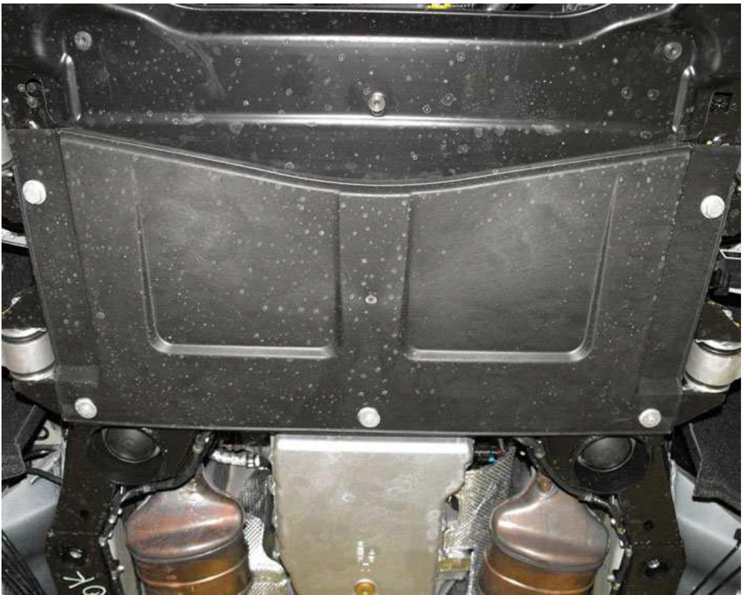
5. Undo the fastening screw and nut (1) and remove the heat guard (2).
