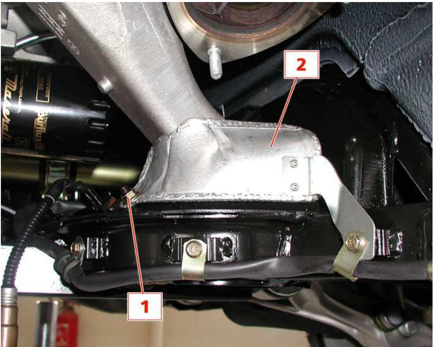
6. Undo the four screws that secure the right-hand side engine mount to the crankcase.
